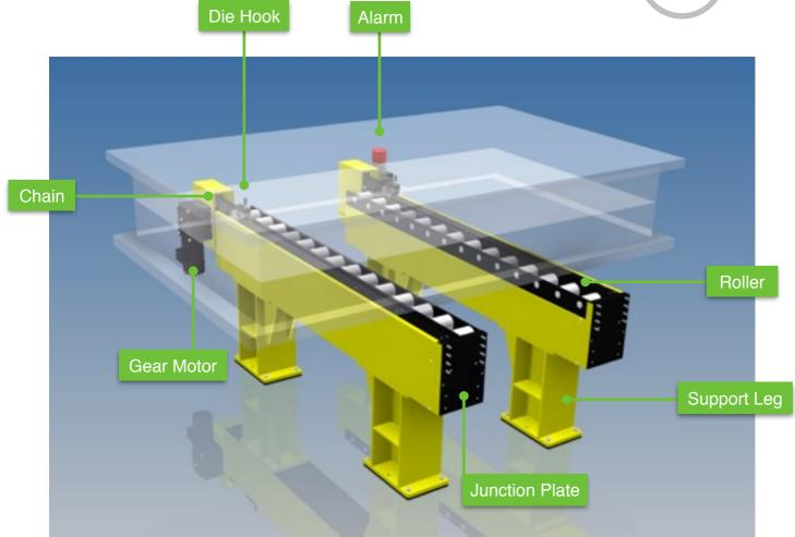
The Powered Bolster Extensions (PBE) is the type of bolster extensions used to transfer the die driven by motor power. The die is connected to the roller chains by die hook. Specially designed roller chains offer great strength to move on the rail.
